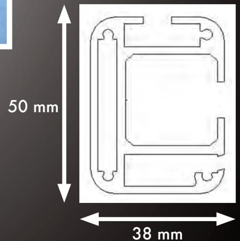
All MSW and MSF systems are provided with standard MSW guides measuring 50 mm. x 38 mm. Triangle and polygonal systems can only be supplied with Soltis 92 / 93 or B 92 N fabric.
