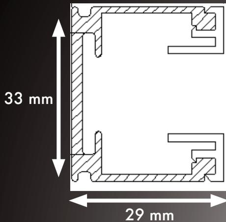
The inner rail and the patented SHY ZIP system are slid into the SHY guide.
