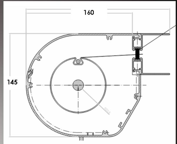
The SZ-MSW 1000 system with ZIP-system is always provided with SZ-MSW guides with measures of 65 mm. x 45 mm. Rectangular systems can be supplied with screen - or acrylic fabric.
